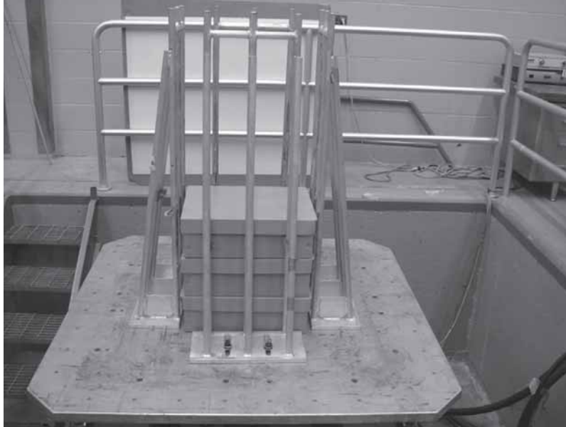
Figure 3. Cantaloupe filled containers packaged in corrugated boxes subjected to random vibration.
