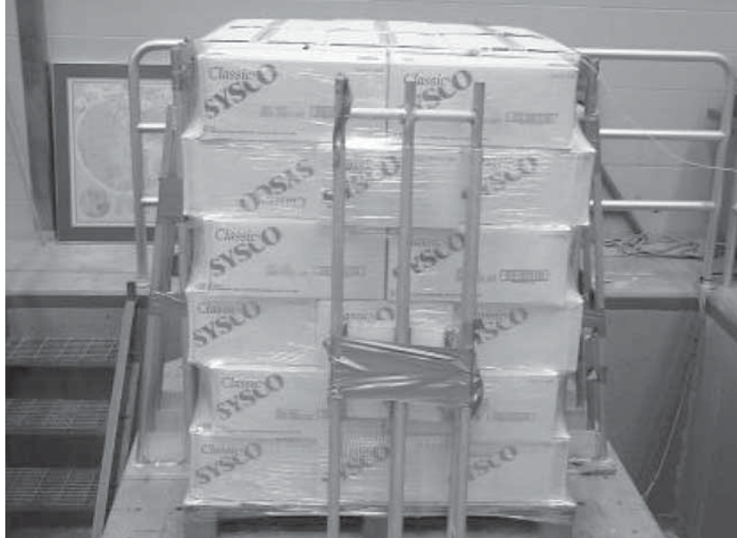
Figure 6. Unitized load of corrugated boxes with steel cans containing juice on BISON pallet.
