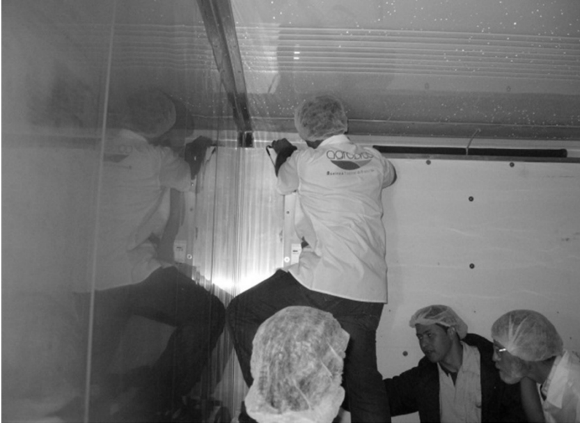
Figure 3. Mounting Temperature Recorder Inside Container.
