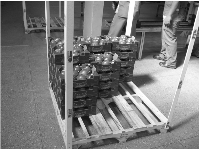
Figure 9. A wood pallet with corner posts being loaded with filled trays.
