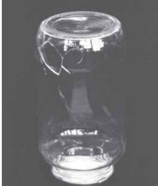
Figure 8. Hydrodynamic breakage situated on the heel of jar with cushion.
