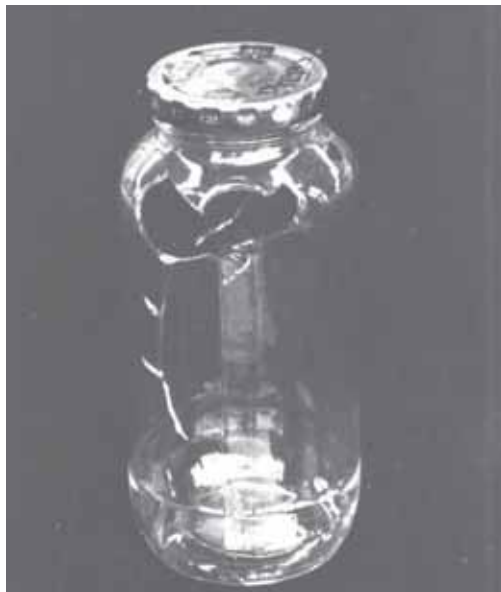
Figure 7. Hydrodynamic breakage located on the shoulder of jar with no cushion.
