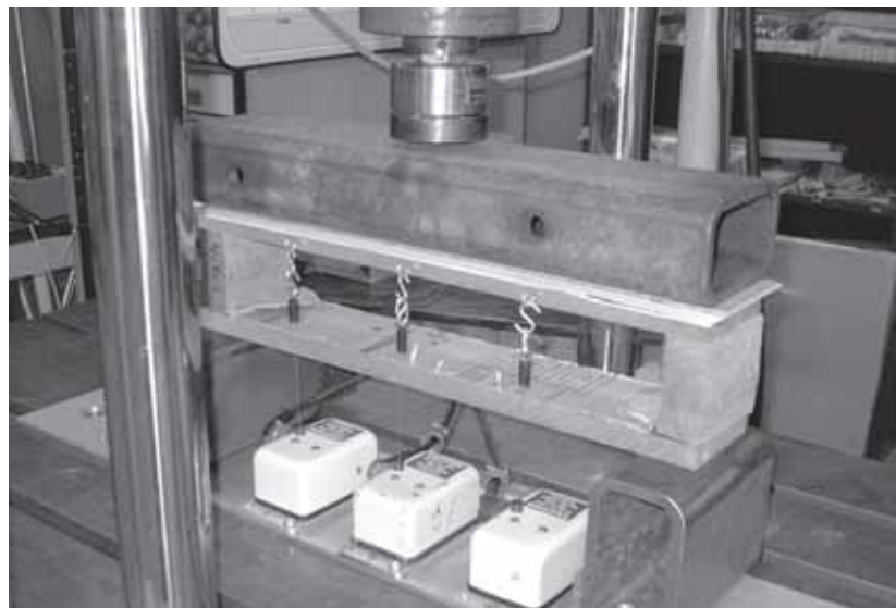
Figure 2. Testing set-up for pallet sample compression.
