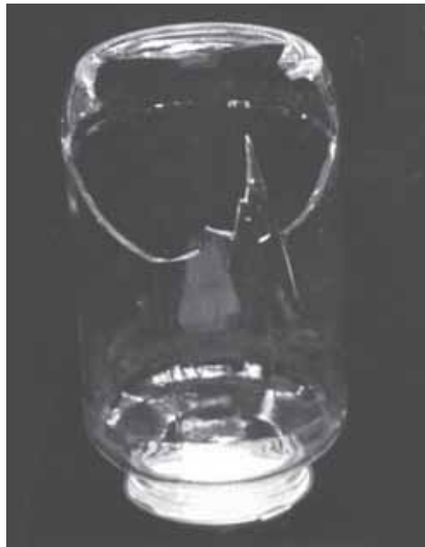
Figure 9. An example of a combination of hydrodynamic breakage and normal point source branching.
