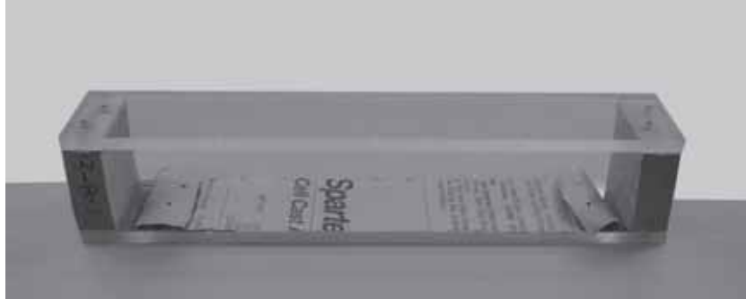
Figure 1. Example of pallet test section sample with Plexiglas® deckboard.
