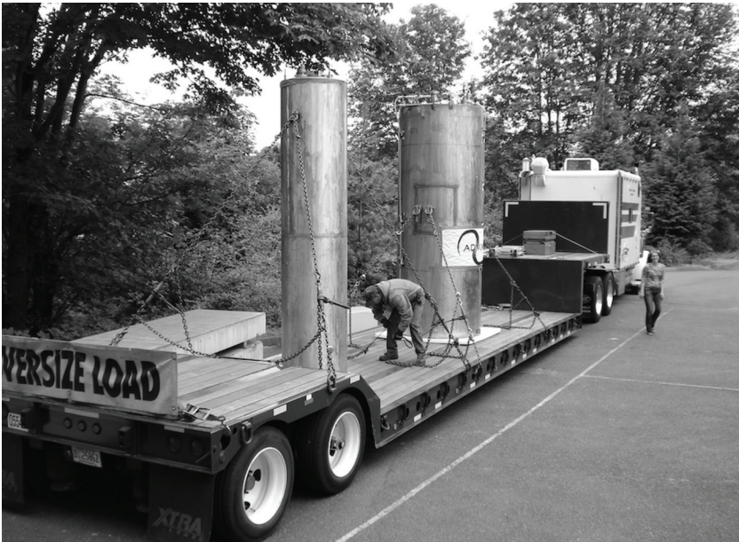
Figure 3. The cryostat and trailer after arriving at the University of Washington. The smaller diameter cylinder in the foreground housed a non-critical experimental apparatus.
