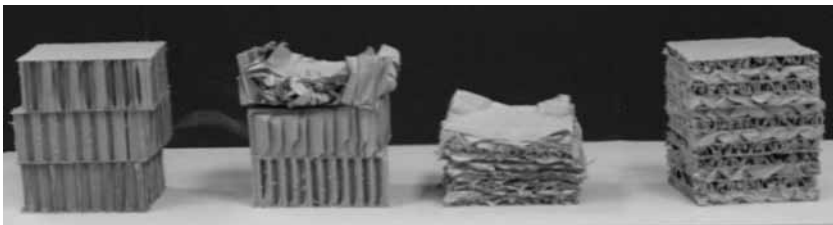
Figure 7. Samples of the Kraft paper folded prismatic structure and the Honeycomb crushed at 40ft/sec impact speed (taken from source [1]).
