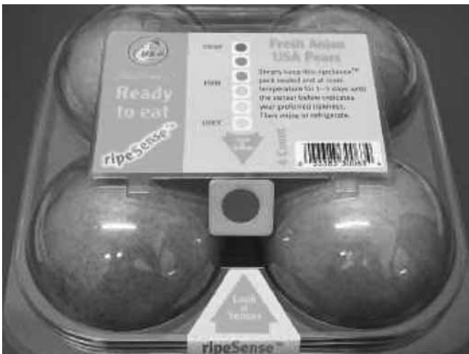
Figure 4. RipeSense™ has a spectrum of colors which designate how ripe the pears are 10 .
