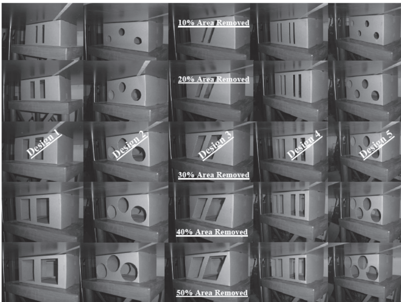
Figure 3. Vent Hole Test Samples.
