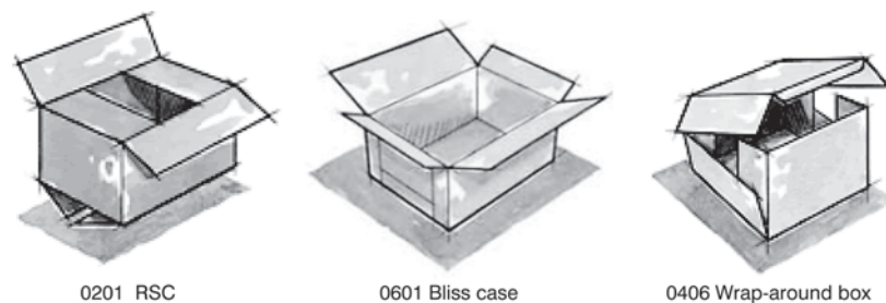
Figure 1. Three styles of the corrugated boxes (drawings are courtesy of Fibre Box Association) [2].
