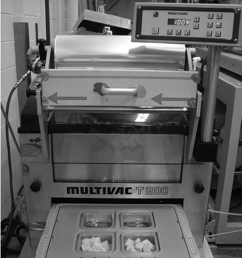
Figure 4. Semi automatic tray sealer (Multivac Model T-200, Inc, Kansas City, MO, USA).
