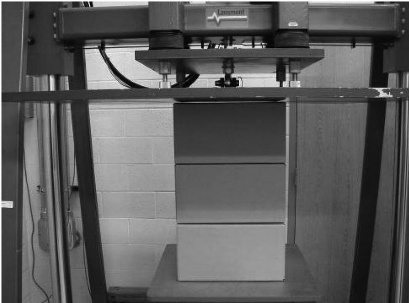
Figure 4. Test setup for misaligned three-high stacks of boxes along the long edge.
