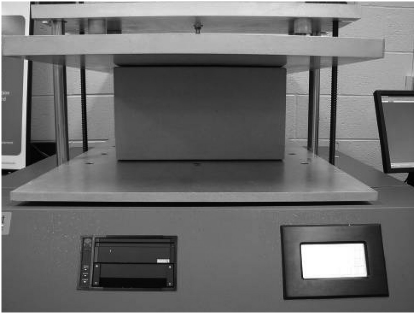
Figure 2. Test set up for single box compression strength.
