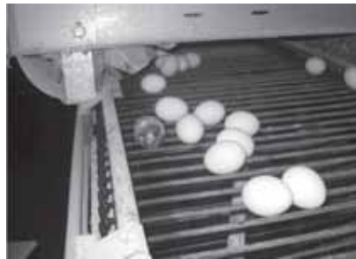
Figure 6. Elevator to Rod Conveyor.
