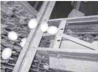
Figure 5. Gathering Belt to Elevator.
