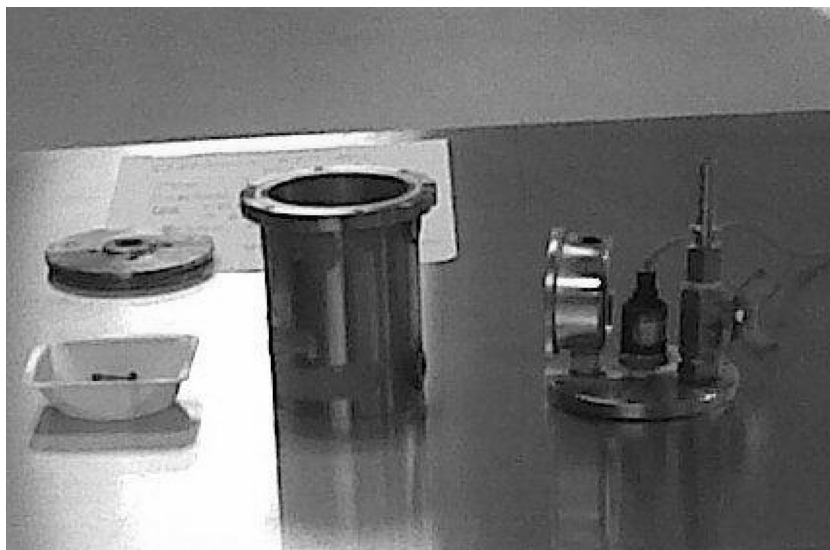
Figure 2. Stainless steel module used to record temperatures at top and bottom during retort processing.
