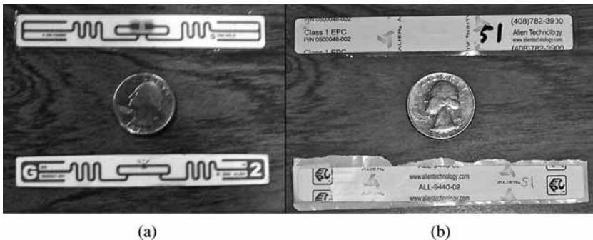
Figure 4. (a) Back of Gen 1 Tag (top) and Gen 2 Tag (bottom). (b) Front of Gen 1 Tag (top) Gen 2 Tag (bottom).
