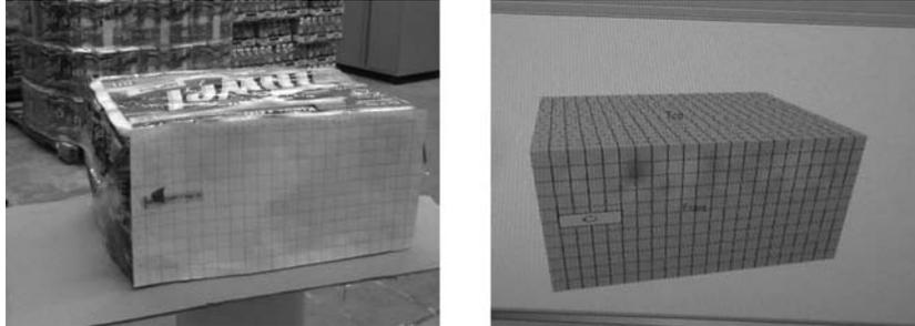
**Figure 3.** Test Setup for Optimum Tag Location Testing in the Horizontal Orientation.
