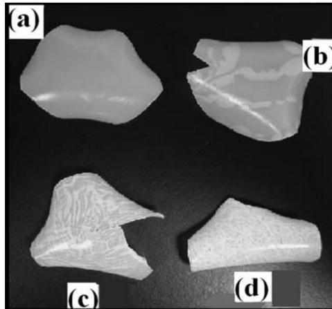
**Figure 2.** Steam-treated PLA: (a) 100°C-4h, (b) 110°C-4h, (c) 100°C-8h, (d) 110°C-8h.
