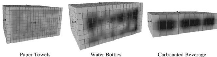
**Figure 5.** RF Performance Comparison of Alien Super Squiggle Tags Placed Horizontally for Products.
