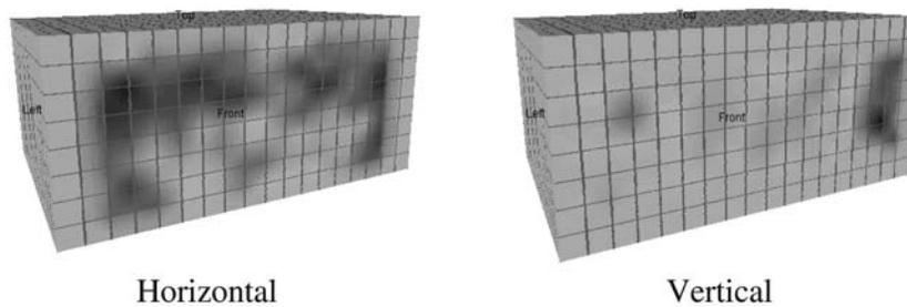
**Figure 4.** RF Performance Comparison of Alien Super Squiggle Tags Placed on Bottled Water Cases.
