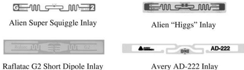
**Figure 2.** RFID Tag Inlays.
