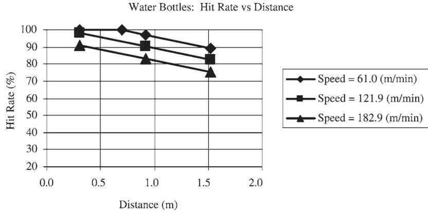
**Figure 7.** Plot of hit rate versus distance over range of test speeds for water bottles.
