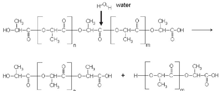
**Figure 5.** Hydrolysis of PLA.
