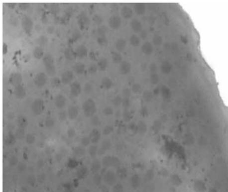
**Figure 3.** Pores in steam-treated PLA 120°C-8h ( $\times 60$ ).
