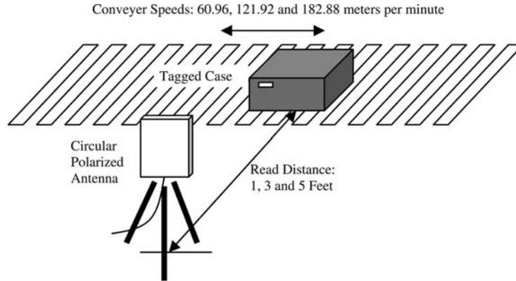
Figure 6. Experimental Setup Deployed for Conveyer Belt Testing.
