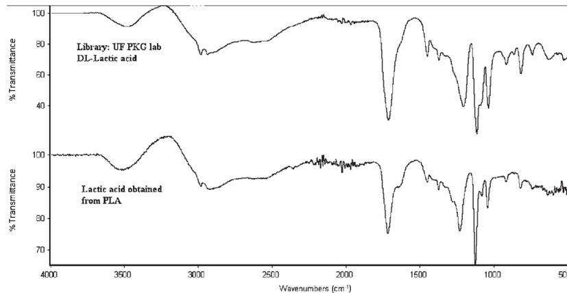
**Figure 9.** Spectra of lactic acid obtained by FTIR-ATR.
