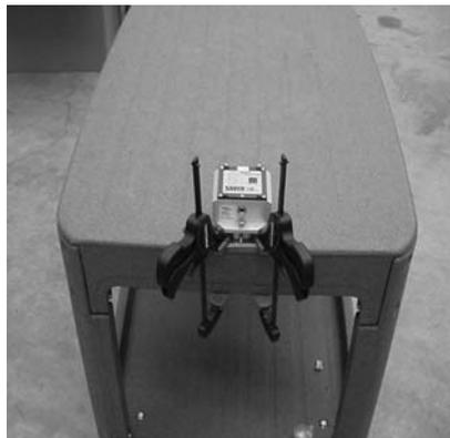
**Figure 2.** Mounting of Recorder on Push Carts.
