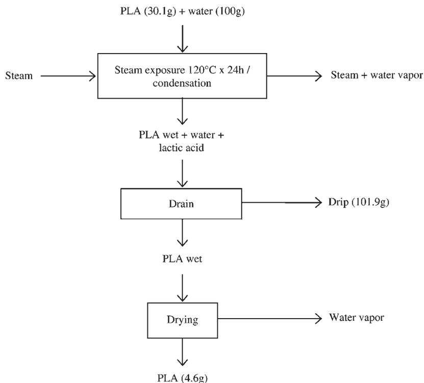
**Figure 8.** Mass balance of PLA treated with steam at extreme conditions.
