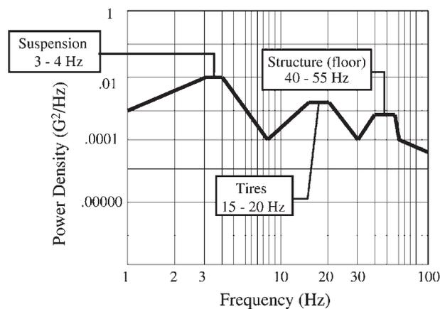
**Figure 1.** A Typical PSD Plot for Truck Transportation.
